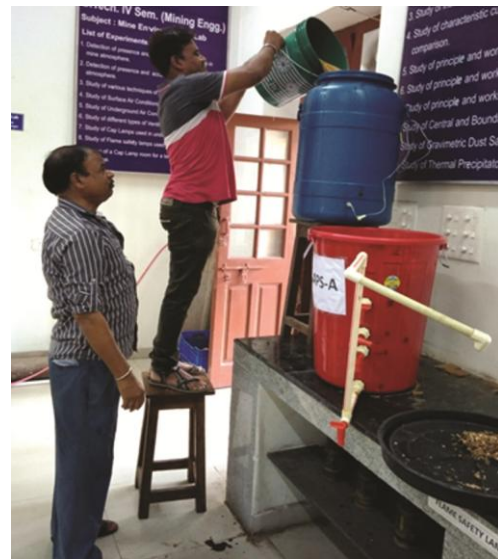
Fig. 3 — Filling of synthetic AMD in influent tank
