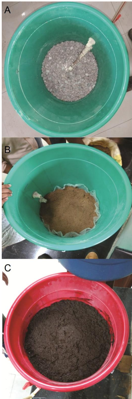
Fig. 2 — (A) Limestone layer filling in Saps unit; (B) Saw dust layer filling in Saps unit; and (C) Cow compost filling in Saps unit
