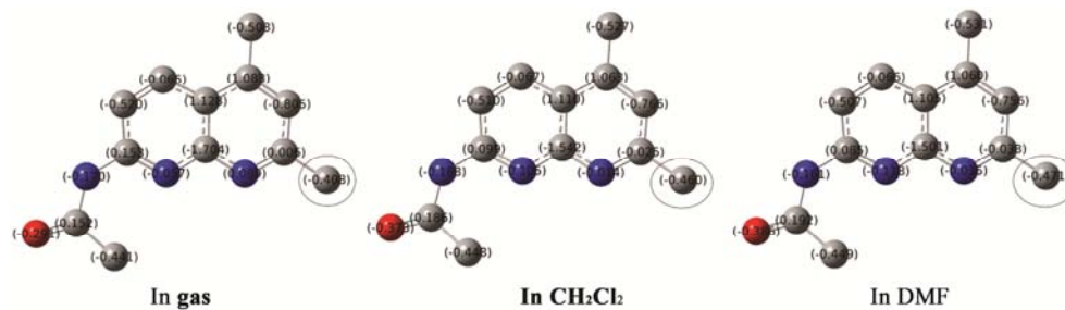
Fig. 3 – DFT optimized structures and atomic charge of 1 at 6-311++G** level in different solvents.
