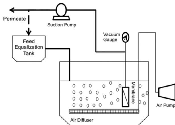
Fig. 1 — Submerged MBR schematic diagram
