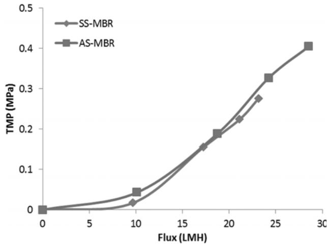
Fig. 5 — Critical Flux test for the hollow fibre membrane module.
