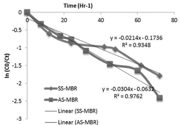
Fig. 4 — The first-order kinetics model for COD reduction
