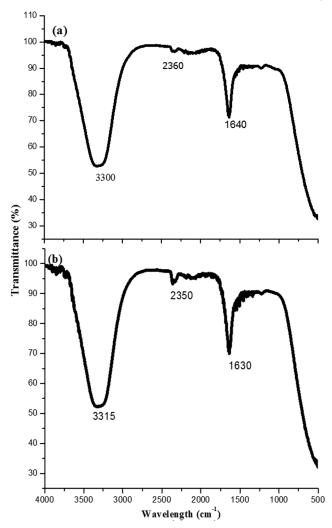
Fig. 3 — (a-b) FT-IR spectra of *Coccinia grandis* flower extract and synthesized Cu nanoparticles.
