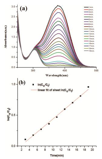
Fig. 4 — (a-b) Absorption spectra of reduction of paranitroaniline using CuNPs as a catalyst in presence of NaBH<sub>4</sub> in aqueous medium and plot of  $\ln |C_0/C|$  versus reduction time.
