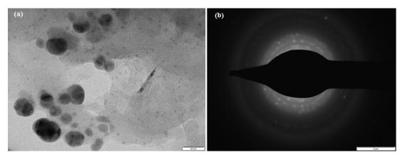
Fig. 1— (a-b) TEM and SAED pattern of the synthesized CuNPs.
