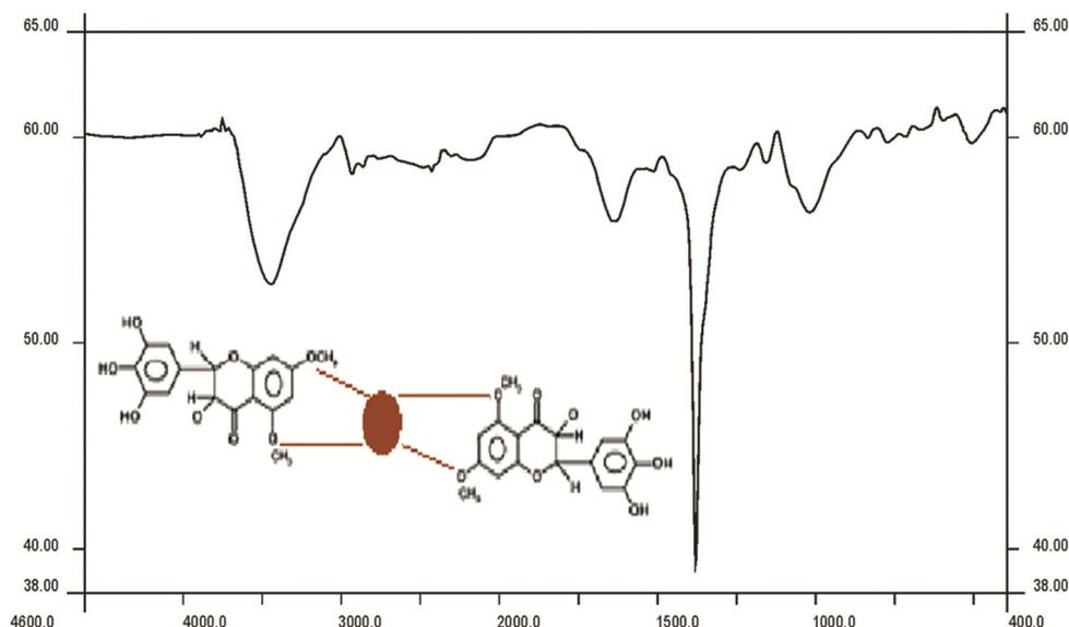
Fig. 4 — FTIR spectra of *Curculigo orchoides* root extract reduced silver nanoparticles.
