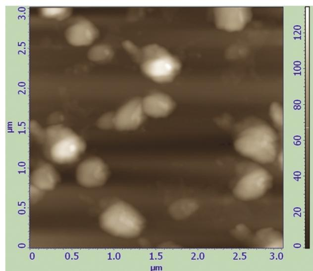
Fig. 5 — AFM image of *Curculigo orchoides* root extract reduced silver nanoparticles.
