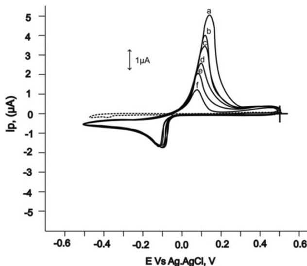
Fig. 3 — Cyclic voltammograms of *Curculigo orchoides* root extract reduced silver nanoparticles. 1mM  $\text{AgNO}_3$  (metal salt) in 0.1M  $\text{KNO}_3$  (supporting electrolyte) at GCE vs Ag/AgCl electrode at scan rate  $10 \text{ mV}\cdot\text{s}^{-1}$ . (a) 1<sup>st</sup> CV cycle just after spiking the root extract; (b to f) subsequent 2<sup>nd</sup> to 6<sup>th</sup> CV cycle.
