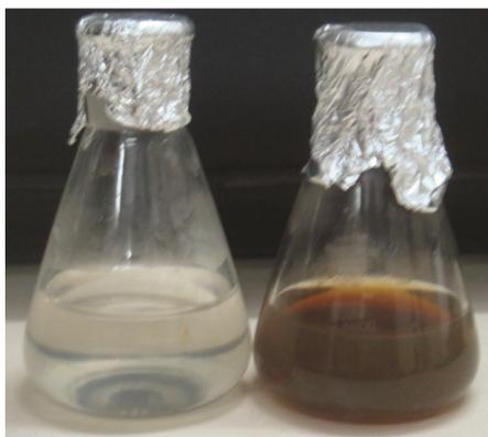
Fig. 1 — Flasks containing 1mM silver nitrate aqueous solution without (A) and with (B) *Curculigo orchoides* root extract (0.2%) after 45 min of reaction.
