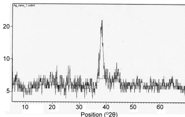
Fig. 6 — XRD pattern of biosynthesized silver nanoparticles.
