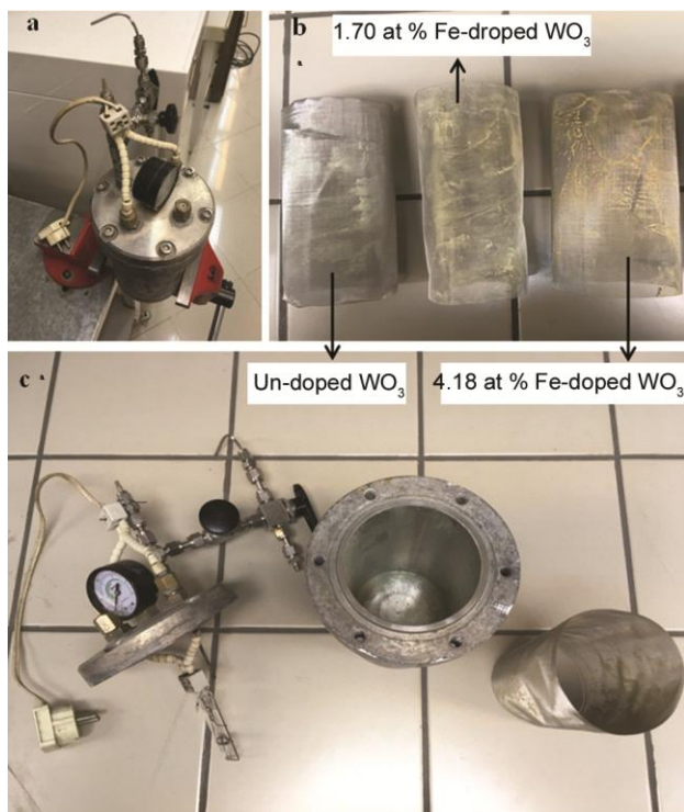
Fig. 1 — The real photographs of (a) assemble photoreactor, (b) coated cylindrical stainless steel webnets with un-doped and Fe-doped \text{WO}_3 nanoparticles (c) open photoreactor with its cap, lamp situation, and also supported catalyst situation in the photoreactor vessel.
