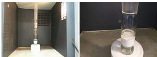
Photo 1 — Microwave reactor with specially designed glass reactor for honey comb reaction.
