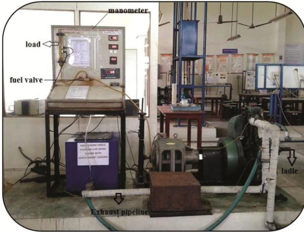
Fig. 3 — Kirloskar four-stroke ICE
