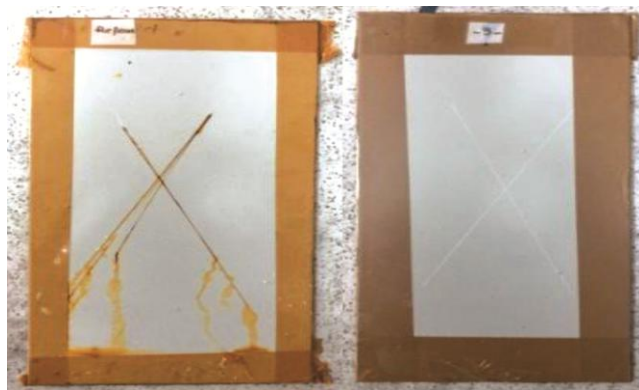
Fig. 3 —Images after 96 hours of reference and optimum plates
