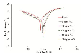
Fig. 2 — Potentio dynamic polarization curves for CS in 0.5 M HCl without and with different concentrations of AO at  $20^{\circ}$ C (immersion time is 60 min).
