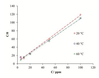
Fig. 8 — Langmuir adsorption isotherm for carbon steel in 0.5 M HCl containing various concentration of AO at 20, 40 and 60  $^{\circ}$ C.
