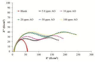
Fig. 3 — Nyquist plots for carbon steel in 0.5 M HCl at  $20^{\circ}$ C in the absence and presence of different concentrations of AO.
