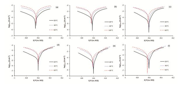
Fig. 5 — Tafel polarization curves of carbon steel in 0.5 HCl M solution at 20, 40 and 60  $^{\circ}$ C in the absence of the inhibitor (a), and in the presence of 5 (b), 10 (c), 20 (d), 50 (e) and 100 ppm (f) of AO.
