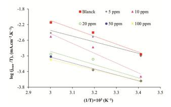
Fig. 7 — Transition-state plots for carbon steel corrosion rates in 0.5 M HCl solution in absence and presence of 5, 10, 20, 50 and 100 ppm of AO.
