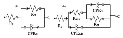
Fig. 4 — The electrochemical equivalent circuit used to fit the data of EIS experiment for the corrosion of carbon steel in 0.5 M HCl solution in theabsence (a) and presence of AO (b).
