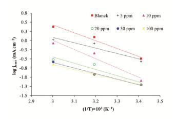
Fig. 6 — Arrhenius plots of A105 carbon steel in 0.5 M HCl medium in the absence and presence of various concentrations of AO.
