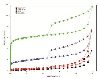
Fig. 2 — Nitrogen adsorption-desorption isotherms of Na-Mt, OH-Al-Mt, CTAB-Mt and CTAB-Al-Mt.
