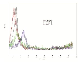
Fig. 1 — XRD patterns of Na-Mt, OH-Al-Mt, CTAB-Mt and CTAB-Al-Mt.
