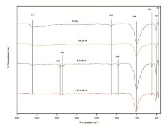
Fig. 3 — FTIR spectra of Na-Mt, OH-Al-Mt, CTAB-Mt and CTAB-Al-Mt.
