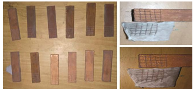
Fig. 11 — Standard tape test results of electroless copper deposited ABS parts for different baths.
