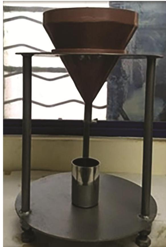
Fig. 1 — New Zealand flow cone apparatus.
