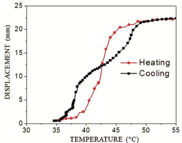
Fig. 2 — NiTi SMA phase Transformations.
