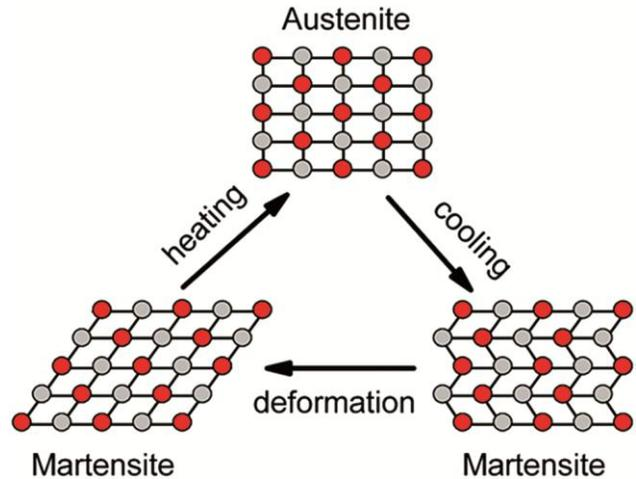
Fig. 1 — SMA phases with its crystal structures.
