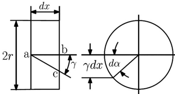
Fig. 3— Cross-section element of Spring.
