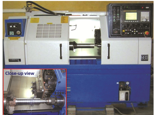
Fig. 2 — CNC Lathe used during machining
