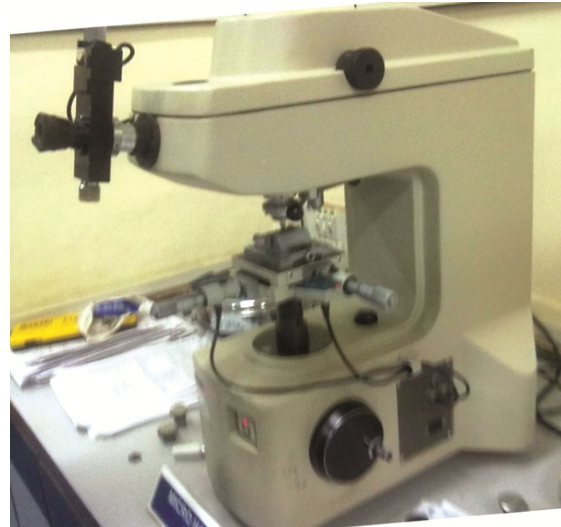
Fig. 4 — Vicker's Micro-Hardness Tester and its Close-up View
