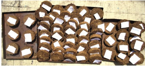
Fig. 2 — Briquettes prepared with cattle dung and pine needle.
