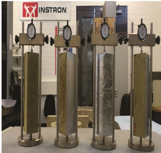
Fig. 6 — Drying shrinkage test setup.
