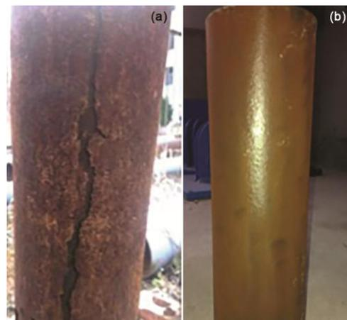
Fig. 11 — Before and after de-rusting of no.3 of group D: (a) Before de-rusting, (b) After de-rusting.
