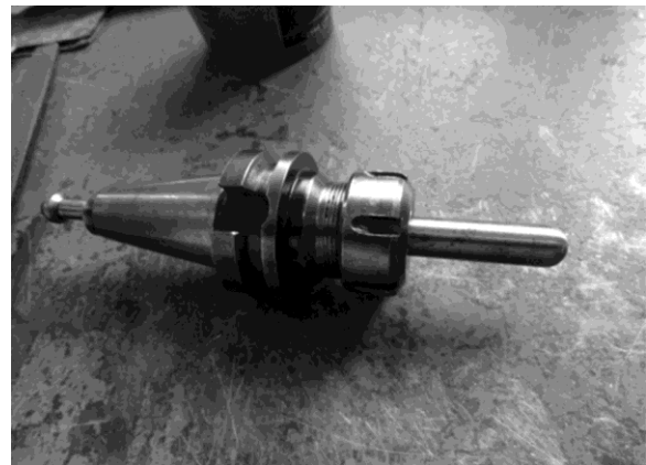
Fig. 2 — K110 steel tool of 20 mm diameter.
