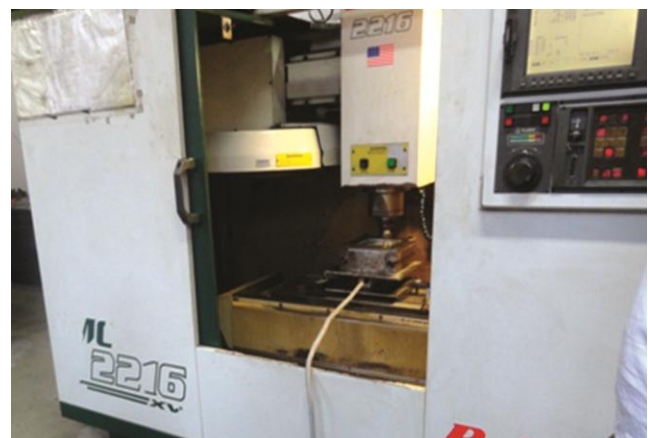
Fig. 3 — Machine tool used for SPIF tests.
