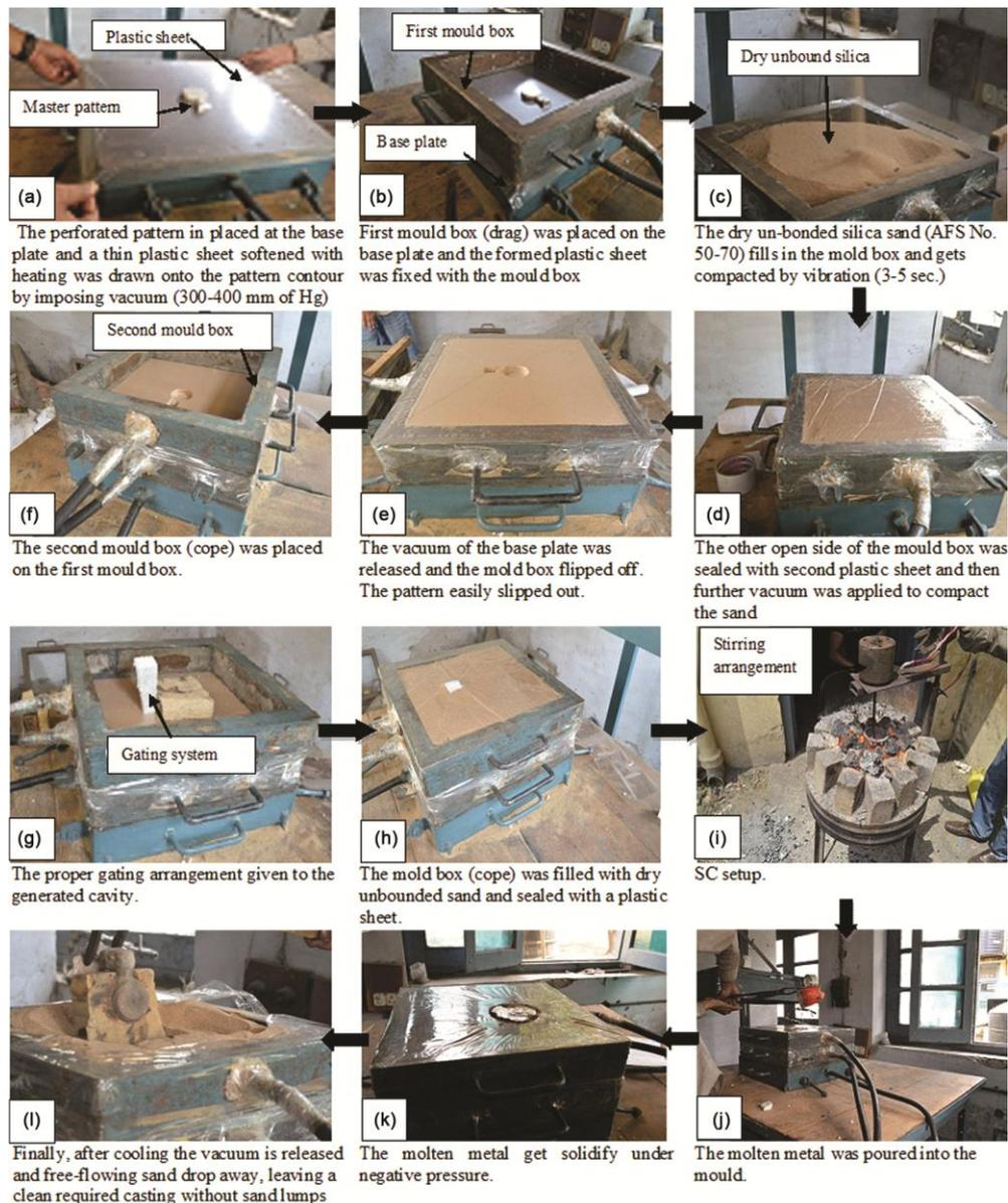
Fig. 2 — Steps for the fabrication Al-AMC using V-process and SC.
