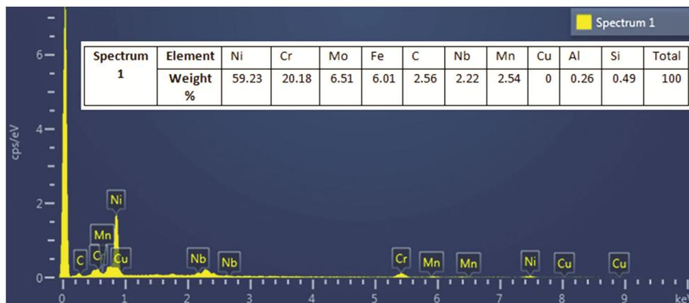
Fig. 5 — Image of the EDS of spectrum 1 of the joint region.
