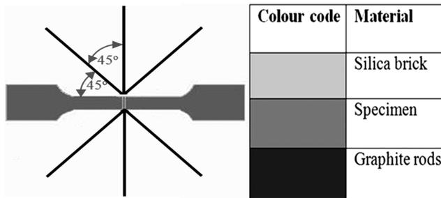
Fig. 3 — Schematic of the top view of the silica brick.
