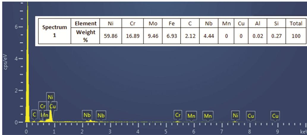
Fig. 2 — Image of the EDS of the original specimen.
