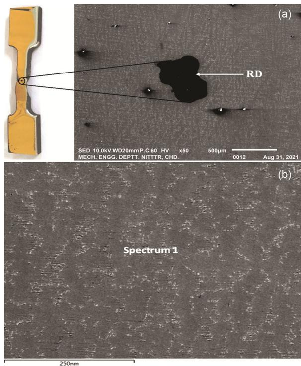
Fig. 4 — (a) Joined specimen with SEM image of the joint zone showing RD, and (b) SEM image of spectrum 1 at the joint.
