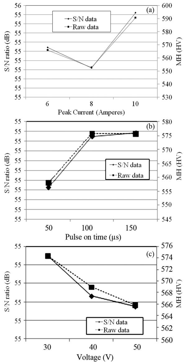
Fig. 6 — Effect on microhardness due to (a) peak current, (b) pulse on time, and (c) voltage.
