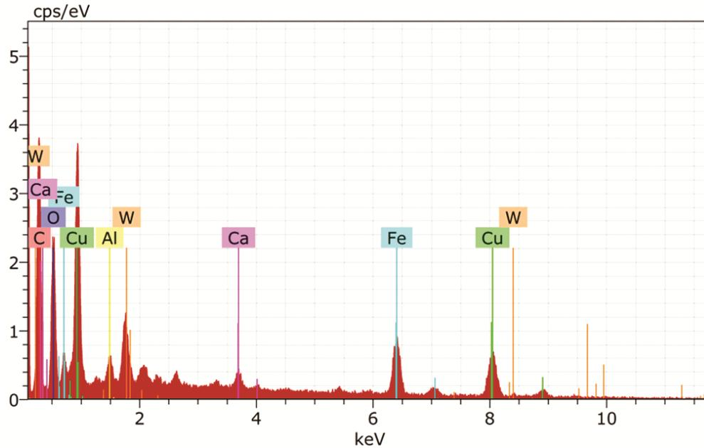
Fig. 10 — EDS spectra of the H11 workpiece machined with Cu-W-CNT electrode.
