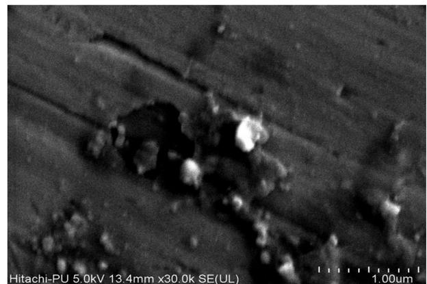
Fig. 1 — FESEM image of H-11 die-steel workpiece.
