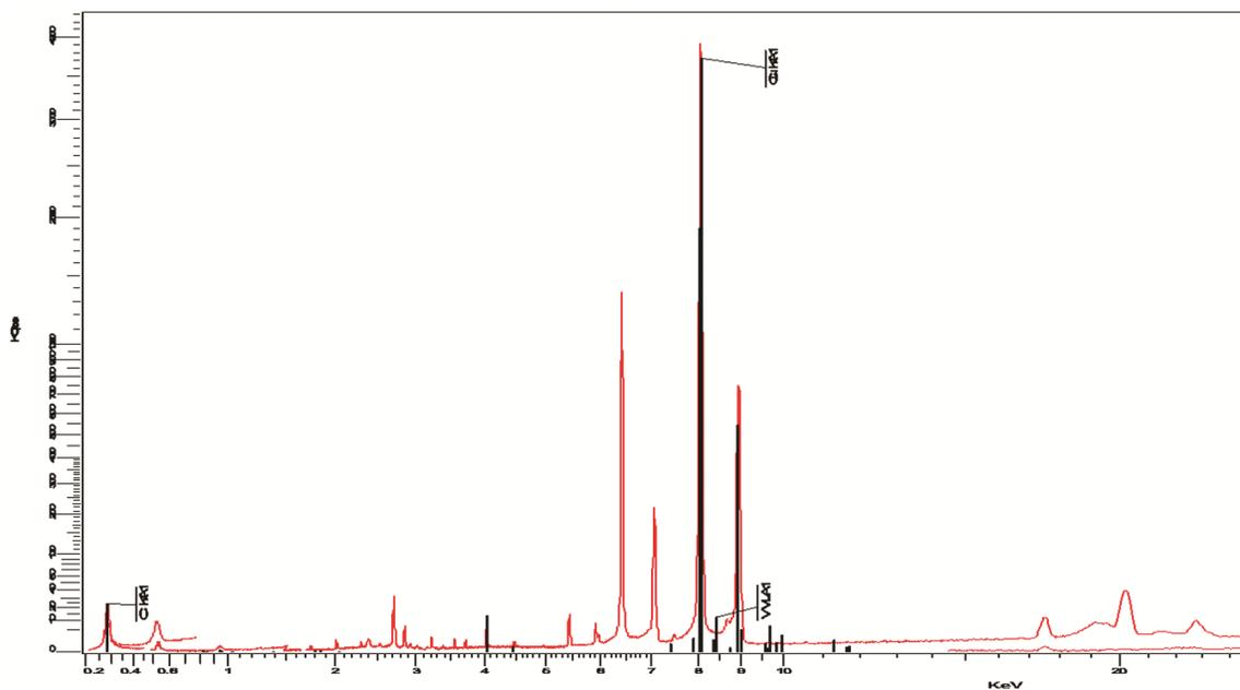
Fig. 4 — WDXRF test of Cu-W-CNT (wt %: 85 - 10 - 05) tool fabricated by Stir casting process.
