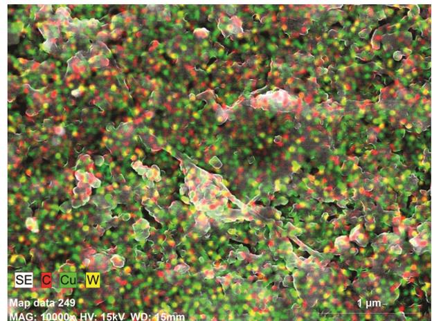
Fig. 9 — Mapping micrograph of the H-11 workpiece.
