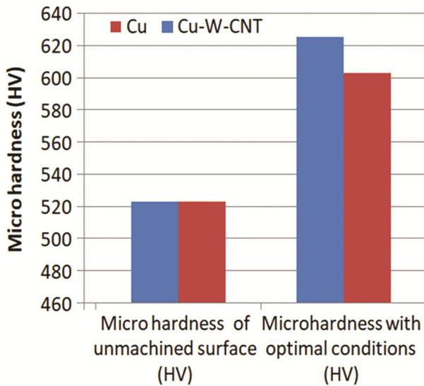
Fig. 7 — Optimal microhardness comparison of the machined surface.
