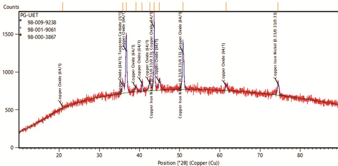
Fig. 11 — XRD pattern of the H11 workpiece machined with Cu-W-CNT electrode.
