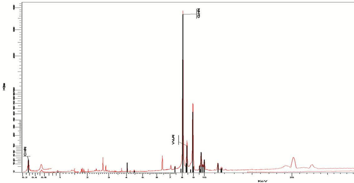
Fig. 3 — WDXRF test of Cu-W-CNT (wt%: 85-10-05) tool fabricated by Powder Metallurgy process.
