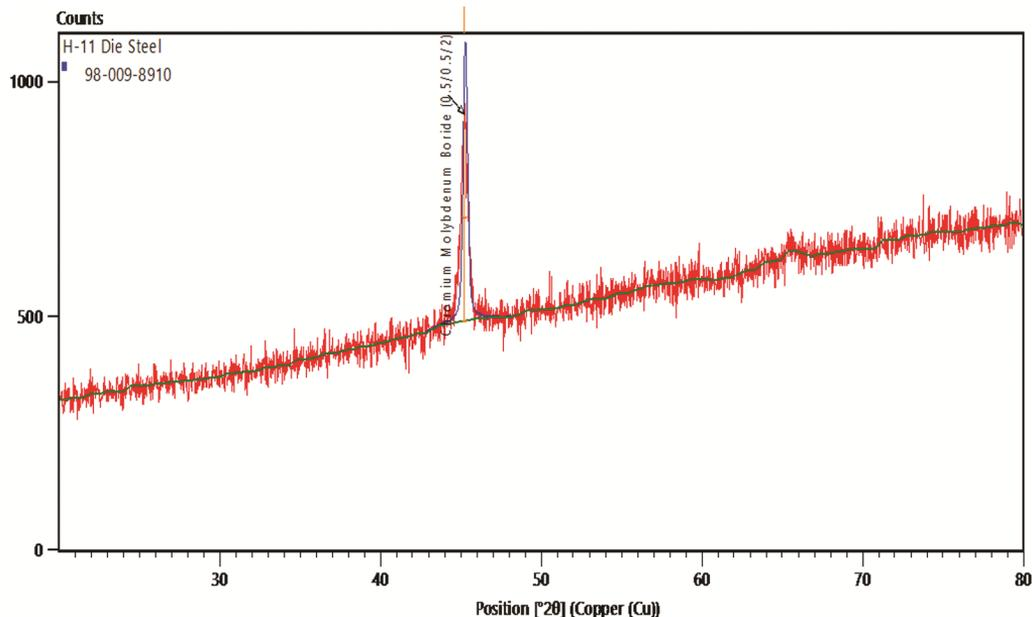
Fig. 2 — XRD results for H11 die-steel workpiece.
