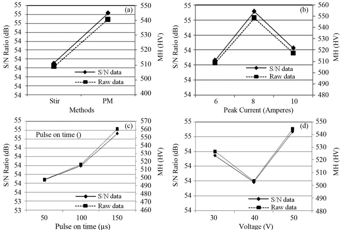
Fig. 5 — Effect on microhardness due to (a) electrode fabrication processes, (b) peak current, (c) pulse on time, and (d) voltage.
