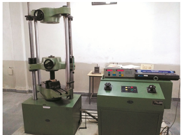
Fig. 4 — Three-point bend test on a particleboard on UTM.
