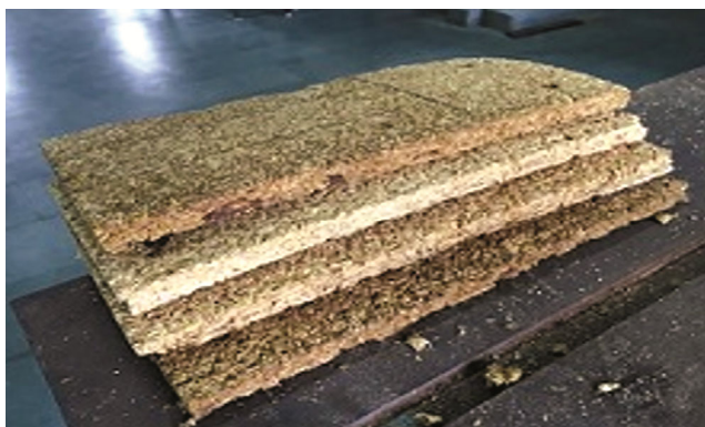
Fig. 3 — Particleboard prepared with rice husk, TA1, and TA2.
