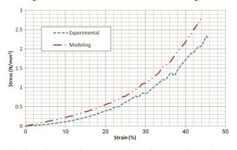
Fig. 6 — Stress-strain curve obtained from experimental and modeling method in state of bias loading
