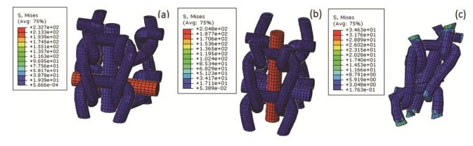
Fig. 4- Stress distribution in fabric unit-cell under (a) course-wise, (b) wale-wise, and (c) bias loading
