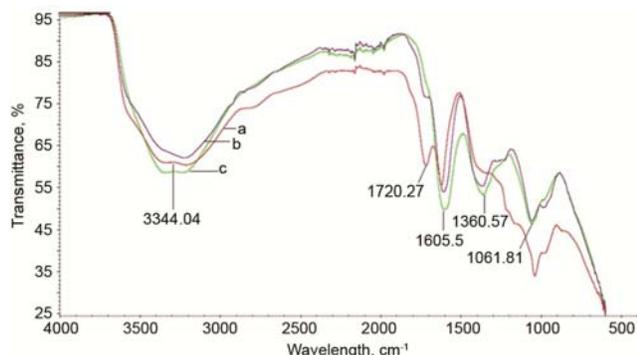
Fig. 1 — FT-IR spectroscopy of reference GO powder before coagulation (a), GO-5-T2 (b) and GO-DA<sub>2</sub>-5-T2 (c)
