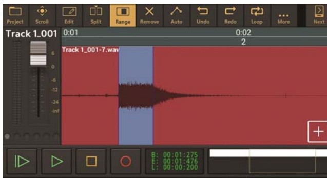
Fig 1 — Valve opening time calculation by sound wave
