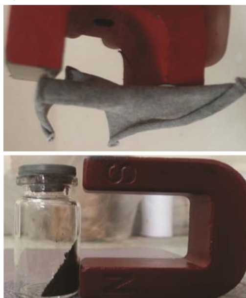
Fig. 5 — Magnetic sensitivity of magnetite powder and treated polyester fabric towards a magnet
