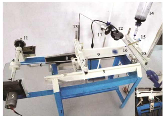
Fig. 1 — A novel device to measure the multi-directional liquid spreading area of stretched fabric [1–base frame, 2–load cell, 3–scale, 4–pulley, 5–dc motor, 6–cord, 7–movable jaw, 8–bearing wheel, 9–fabric sample, 10–fixed jaw, 11–u slot sensor, 12–camera, 13–support stand, 14–water reservoir, 15–drop flow rate controller, 16–syringe]
