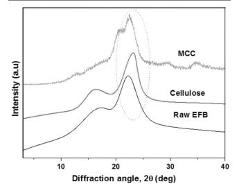
Fig. 4 — XRD profiles of REFB, cellulose and MCC
