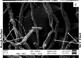
Fig. 3 — SEM micrographs of (A) REFB, (B) cellulose and (C) MCC
