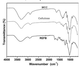
Fig. 2 — FTIR spectrum of REFB, cellulose and MCC
