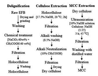
Fig. 1 — Delignification, cellulose extraction and MCC preparation processes
