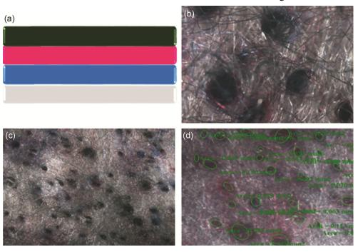
Fig. 2 — (a) Layering sequence of layers, (b) presence of different colours on bottom most layer after punching, (c) number of holes and (d) area covered by the holes
