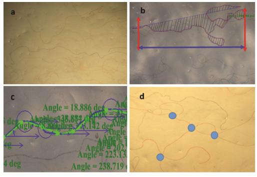
Fig. 1 — (a) Tracer fibre content -0.3%, (b) fibre extent and area covered by fibre, (c) measurement of fibre inclination angle, and (d) cross-over point
