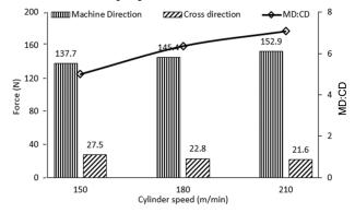
Fig. 4 — Influence of cylinder speed on tensile strength of nonwoven
