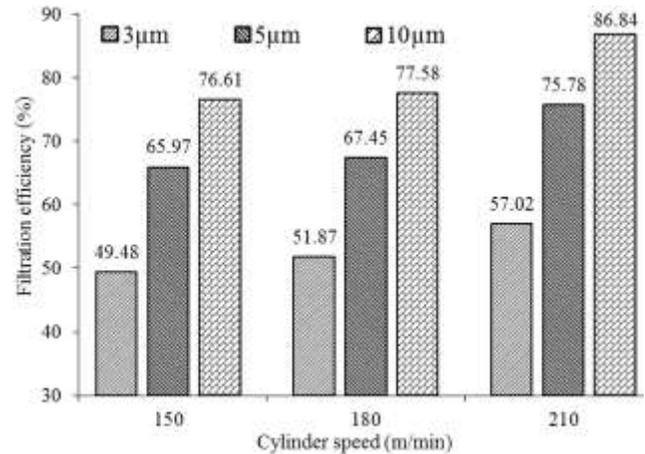
Fig. 3 — Relation between cylinder speed and filtration efficiency
