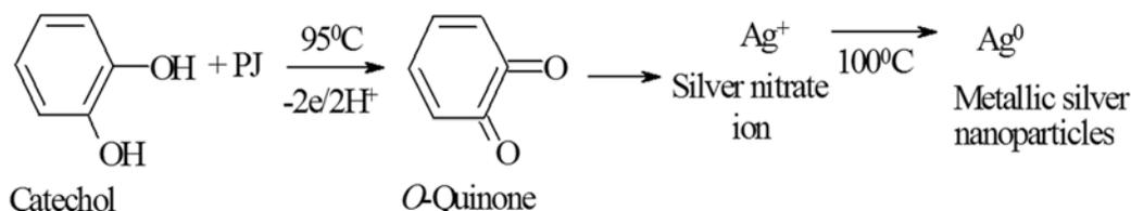
Fig. 2 — Schematic diagram showing synthesis of silver nanoparticles by melanin
