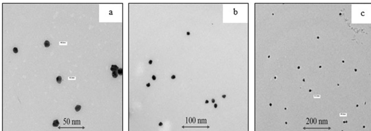
Fig. 3 — TEM images of silver nanoparticles recorded at different magnifications (a)  $\times 50,000$ , (b)  $\times 2,50,000$  and (c)  $\times 520,000$
