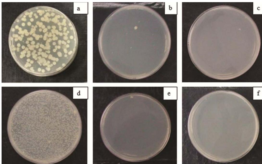
Fig. 6 — Antimicrobial testing of nanosilver treated wool against *S. aureus* (a) control (b) 150 ppm and (c) 200ppm; and against *E.coli* (d) untreated, (e) 150ppm and (f) 200ppm
