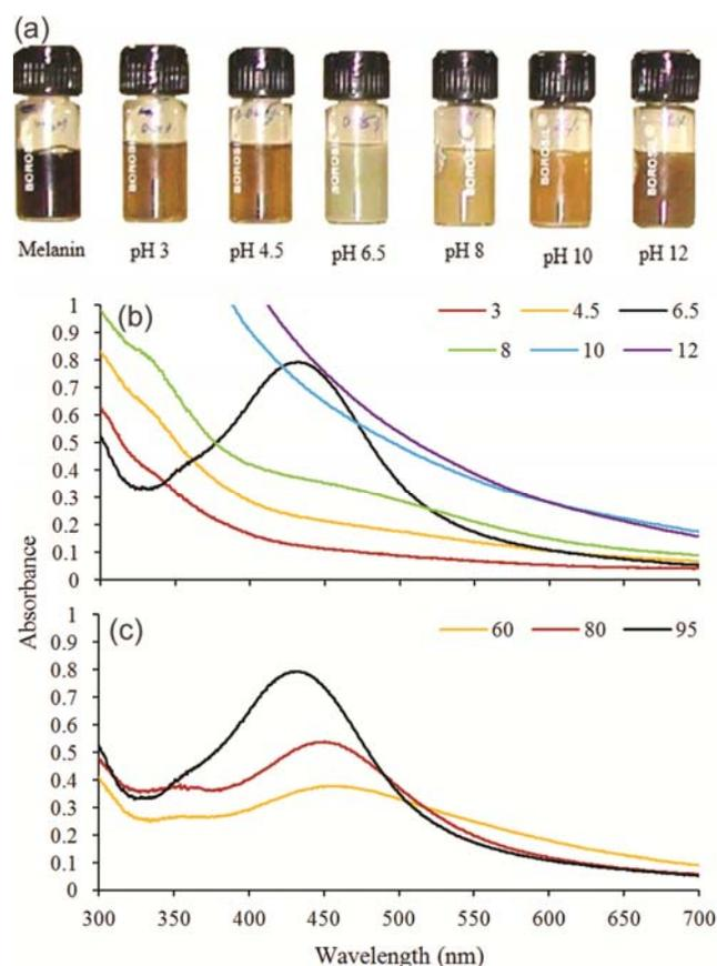
Fig. 1 — (a) Silver nitrate solutions reduced with melanin synthesized at different pH, (b) UV vis spectra of silver nitrate solutions reduced with melanin synthesized at varying pH (0.1% catechol, 25% PJ, 95°C), and (c) effect of temperature on formation of silver nano particles (0.1% catechol, 25% PJ, pH 6.5)
