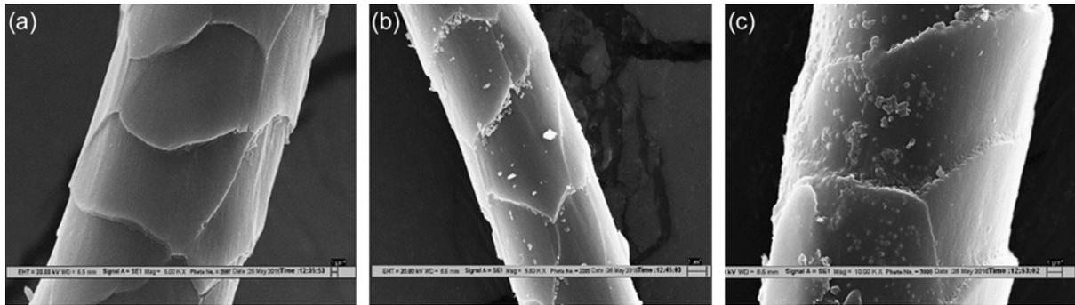
Fig. 5 — SEM images of (a) untreated, and treated with (b) 150 ppm and (c) 200 ppm nanosilver
