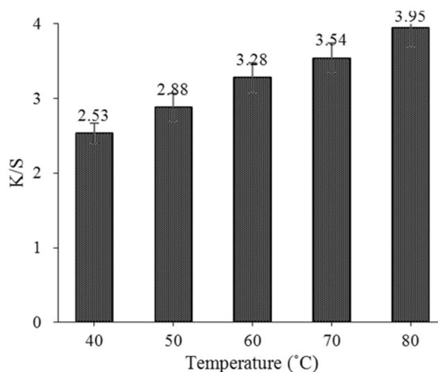
Fig. 4 —  $K/S$  of wool treated with silver hydrosol at different temperature (pH 3)
