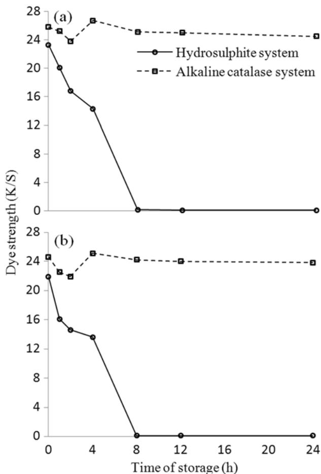
Fig. 3 — Stability of dye baths in (a) absence and (b) presence of dye
