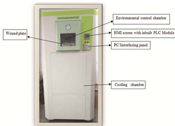
Fig. 2 — SITRA fluid handling capacity tester (SFHCT)
