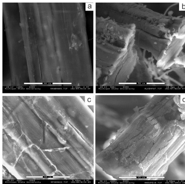
Fig.2 — Images displaying ESEM micrographs of (a) untreated ( $\times 1200$ ), (b) alkali treated ( $\times 900$ ), (c) silane treated ( $\times 900$ ), and (d) acrylonitrile treated ( $\times 1000$ ), hemp fibre<sup>22</sup>
