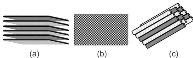
Fig. 6 — Three different types of configurations in which two fibres can be placed in a hybrid composite (a) interlayer, (b) intralayer and (c) intimate mix (redrawn on the basis of Swolfs *et. al.*<sup>42</sup>)
