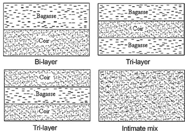
Fig.7 — Different layering patterns and dispersion of fibres reported in coir/bagasse hybrid biocomposites<sup>113</sup>
