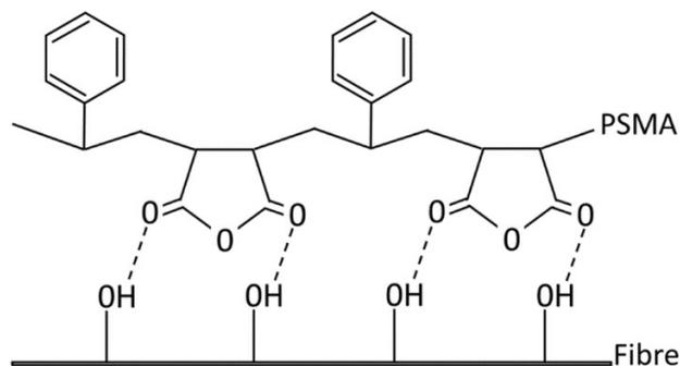
Fig.3 — Proposed model of interaction of polyester and PSMA treated fibre (redrawn on the basis of Idicula *et al.*<sup>60</sup>)
