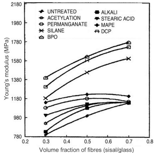
Fig.4 — Effect of various chemical treatments on Young's modulus of sisal/glass hybrid biocomposites at varying fibre ratios<sup>21</sup>
