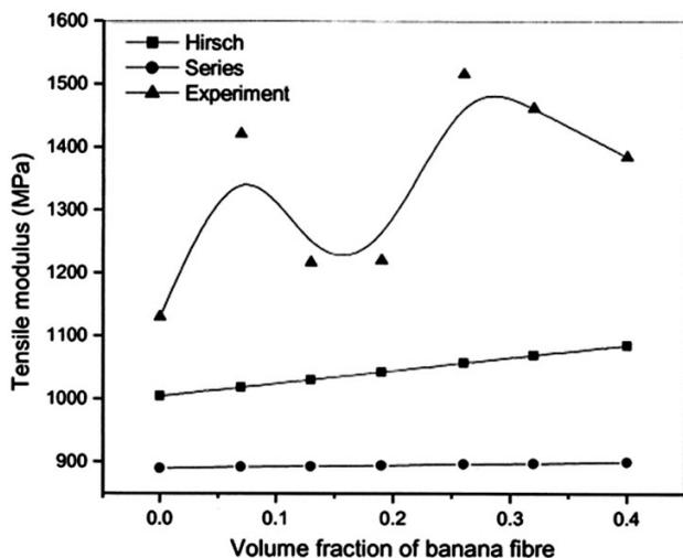
Fig. 8 — Experimental values of tensile modulus of sisal-banana fibre hybrid biocomposites alongwith theoretical models<sup>7</sup>
