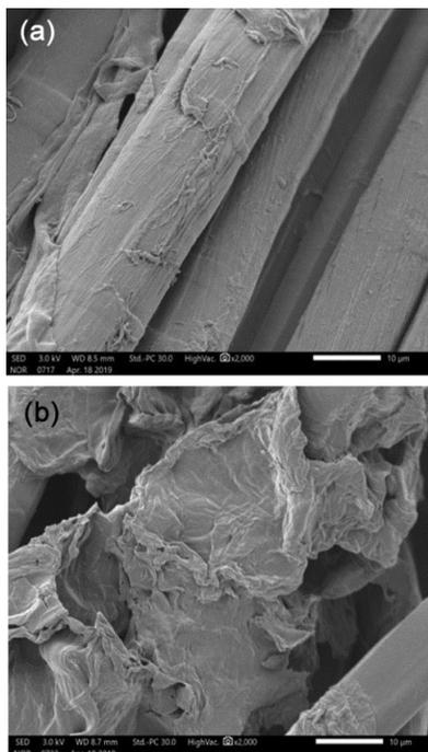
Fig. 2 — SEM images of (a) untreated crosslinked and (b) plasma-treated crosslinked linen fabrics
