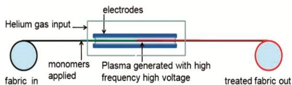
Fig. 1 — Schematic of plasma machine
