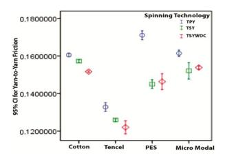
Fig. 6 — 95 % confidence interval graphs for yarn-to-yarn friction coefficients of TPY, TSY and TSYWDC
