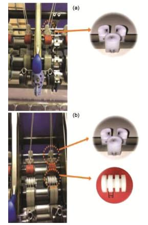
Fig. 1 — (a) Three-strand yarn – TSY and (b) three-strand yarn with delivery cylinder – TSYWDC
