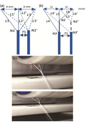
Fig. 5 — Changes in the geometry of spinning triangles during production for TSYWDC (a), and TSY (b), respectively (N= yarn formation point, L= strand length, S= strand space, T= displacement for yarn formation point), fibre loss caused from non-stationary spinning for TSYWDC (c), and two yarn formation points for TSY (d)
