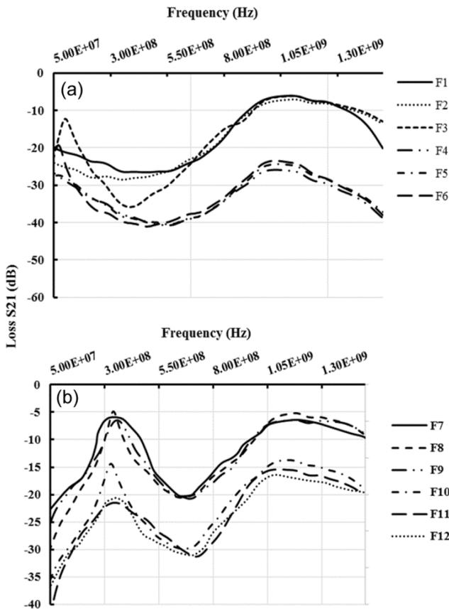
Fig. 4 — Shielding behaviour of different fabrics (a) cell type and (b) plain fabric with different thread patterns
