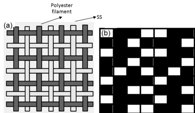
Fig. 2 — Weave patterns used in fabric production (a) plain weave 1p/1m, and (b) cell type weave
