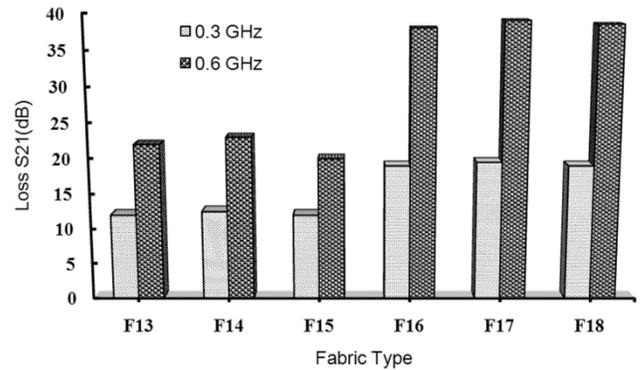
Fig. 5 — Shielding behaviour of plain fabrics at different frequencies
