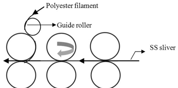
Fig. 1 — Drafting device of ring frame
