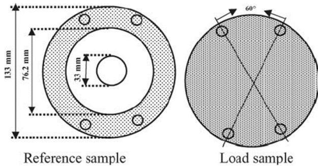
Fig. 3 — Sample holder and required specimens as per ASTM D4935-99 (ref. 1)
