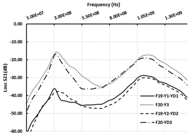
Fig. 6 — Comparison of shielding behaviour of plain and cell type fabrics
