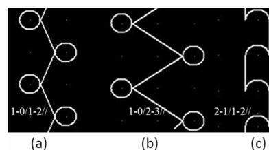
Fig. 1—Three-stitch technology of looped jacquard weave [ (a) 1-0/1-2//, (b) 1-0/2-3// and (c) 2-1/1-2// ]
