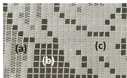
Fig. 2—Three corresponding fabric textures of the weaves in Fig. 1 [ (a) texture 1 region, (b) texture 2 region and (c) texture 3 region ]
