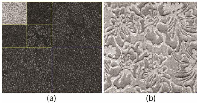
Fig. 4—Pyramidal wavelet decomposition of the jacquard fabric image
