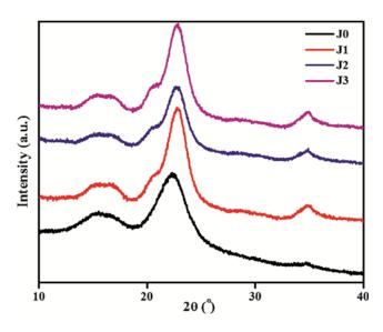
Fig. 3 — Wide angle X-ray diffraction pattern of raw jute sticks (J0) and microcrystalline cellulose produced through 0.5% (J1), 0.7% (J2) and 1.0% (J3) sodium chlorite as delignifying agent
