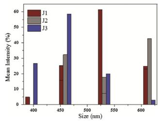
Fig. 2 — Particle size of jute sticks treated with 0.5% (J1), 0.7% (J2) and 1.0 % (J3) sodium chlorite concentration
