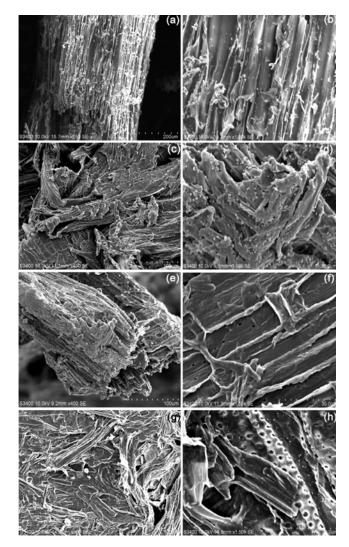
Fig. 5 — SEM images of (a) and (b) jute sticks (J0), and microcrystalline cellulose obtained after treating with three different concentrations (c) and (d) 0.5 % [J1], (e) and (f) 0.7% [J2] and (g) and (h) 1.0% [J3] of sodium chlorite at different magnifications
