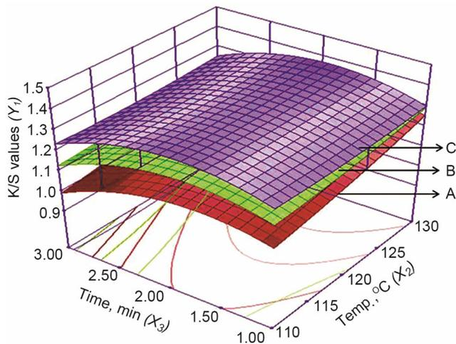
Fig. 3—Response surface plots for the *K/S* values (Y<sub>1</sub>) versus temperature and time at different GTA concentrations (A—10mL/L, B—20mL/L, and C—30mL/L)
