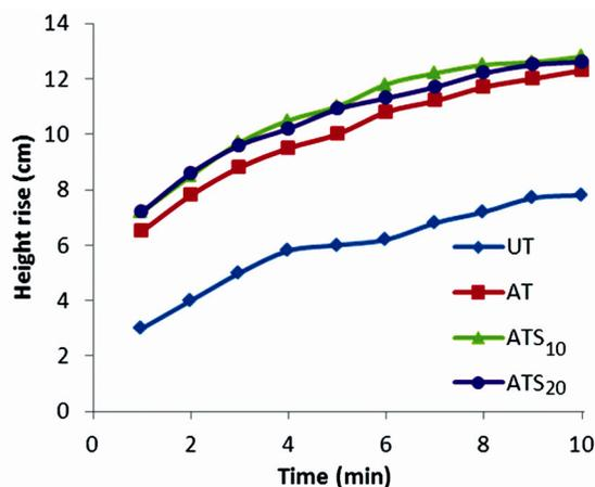
Fig. 6—Vertical wicking values of control and sericin treated polyester (UT–control, AT– alkali treated, ATS<sub>10</sub>– alkali and 10gpl sericin, ATS<sub>20</sub>– alkali and 20gpl sericin)
