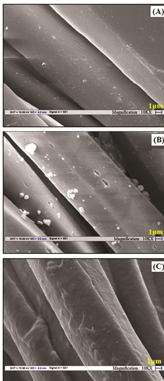
Fig. 1—SEM images of polyester (A) control, (B) alkali treated and (C) treated with alkali and 10g/L of sericin
