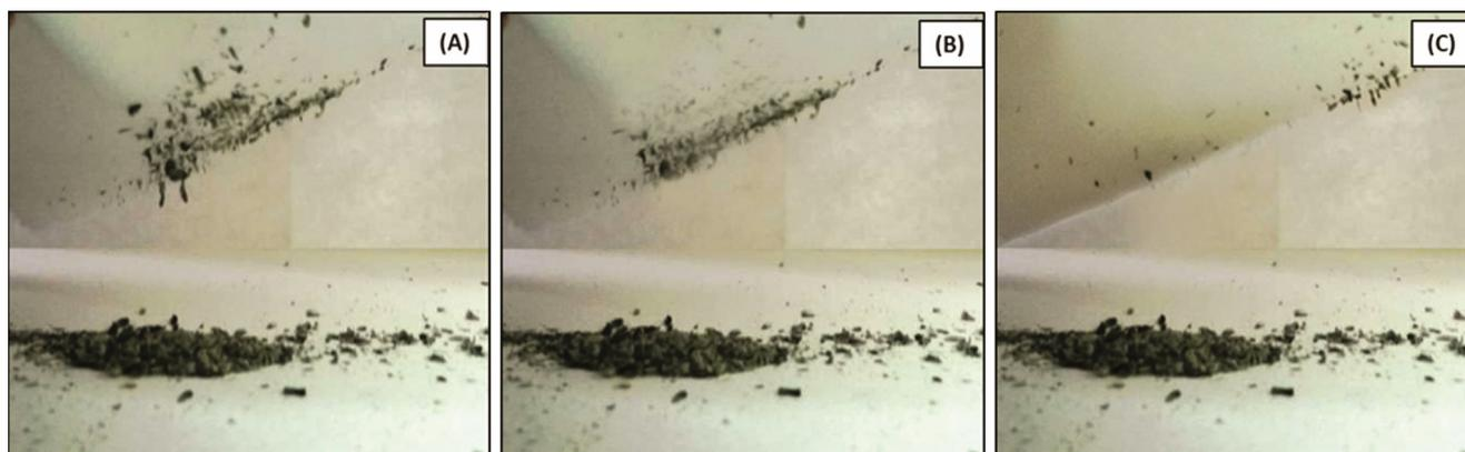
Fig. 7—Ash test for assessment of antistatic property (A) control, (B) alkali treated, and (C) alkali and 10g/L of sericin treated
