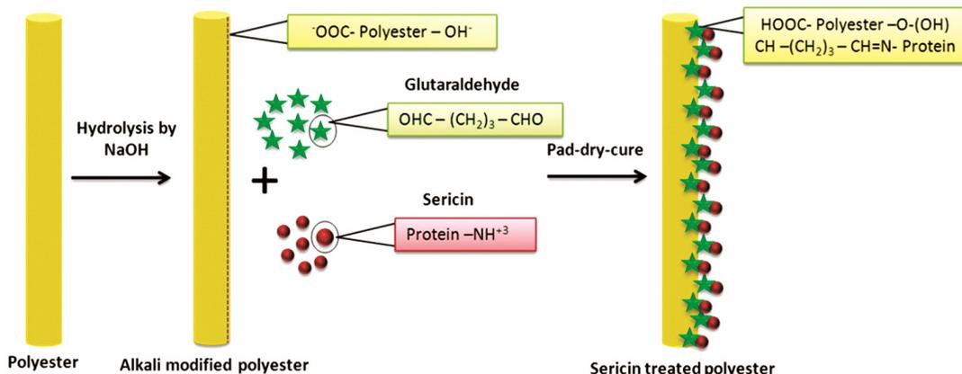
Fig. 4—Graphic representation of sericin application on modified PET using GTA
