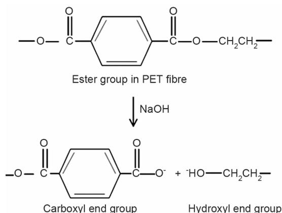
Fig. 2—Alkali hydrolysis of polyester<sup>15</sup>
