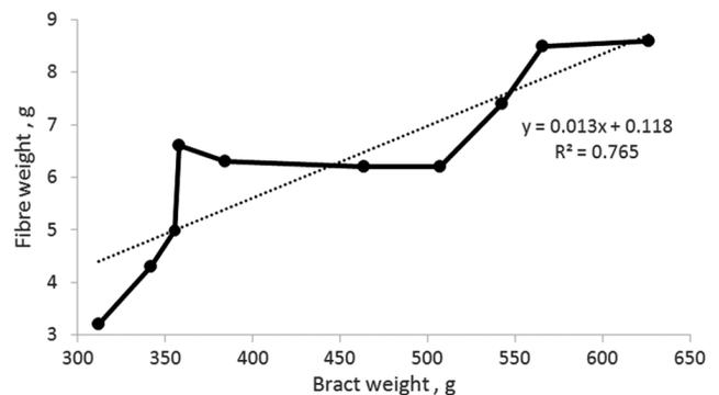
Fig. 1 — Effect of banana bract weight on fibre weight
