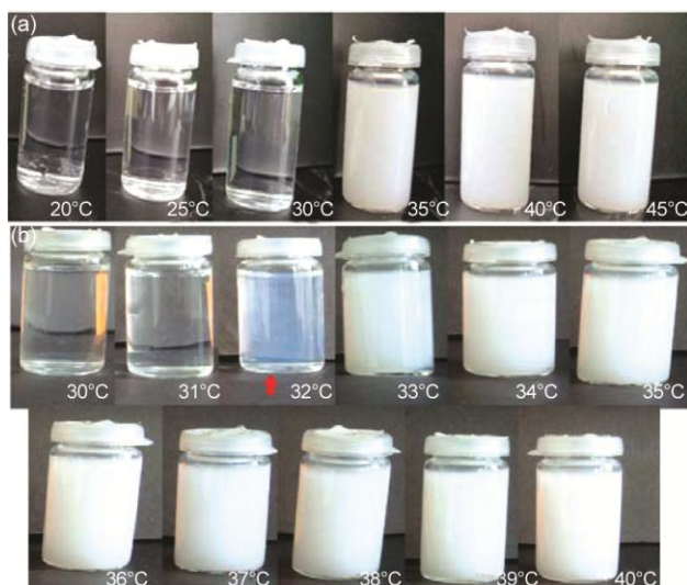
Fig. 3 — Thermo-responsive behavior of PNIPAM polymer solution (a) at 20–45 °C (with 5 °C increment) and (b) at 30–40 °C (with 1 °C increment)
