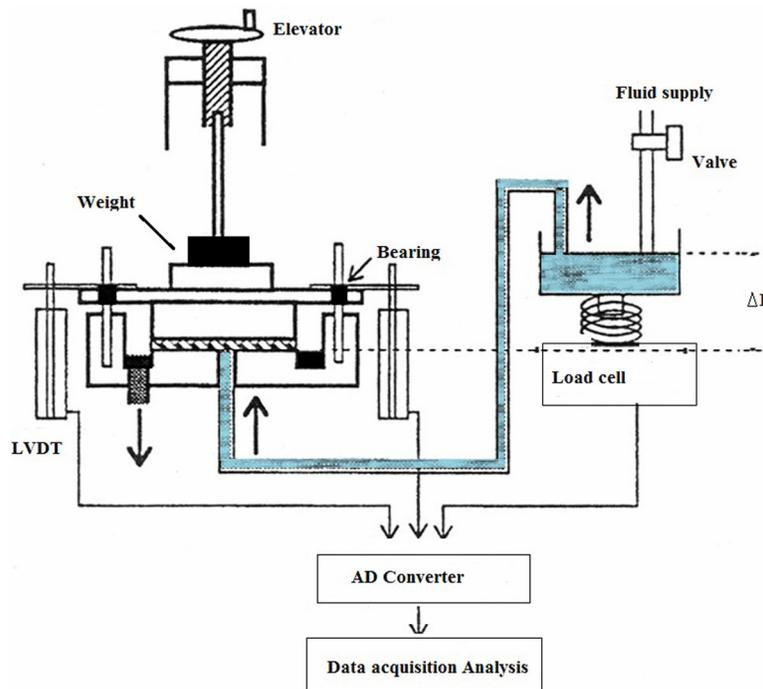
Fig.3 – Components of gravimetric absorbency tester (GATS)
