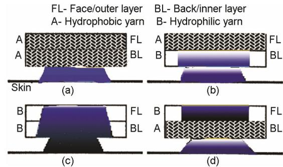
Fig.2 – Double layer fabrics with different water absorbability in face and back layers<sup>23</sup>
