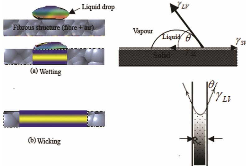
Fig. 1 – Wetting and wicking phenomenon in textile structures<sup>10</sup>
