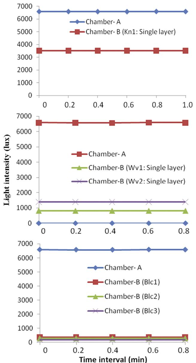
Fig.2 — Light cutting ability of different fabrics
