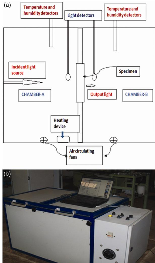
Fig.1 — (a) Line diagram of instrument and (b) photograph of instrument to determine heat and light cutting ability of curtain
