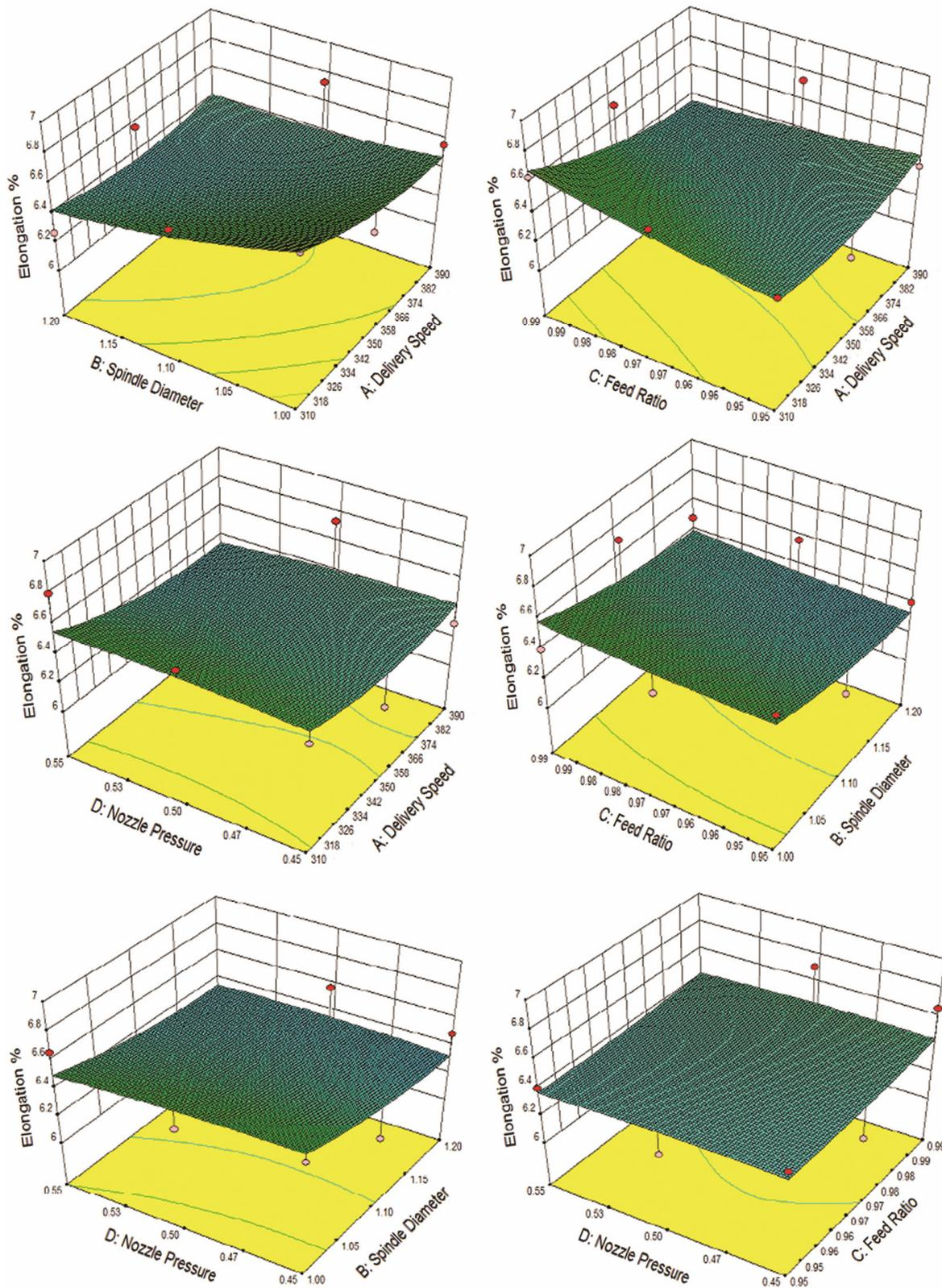
Fig. 4 — Interaction of spinning parameters on elongation of Ne 40 polyester/cotton vortex yarn
