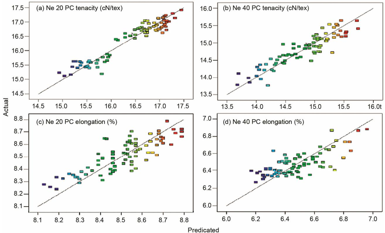
Fig. 5 — Predicted versus observed values of tenacity and elongation of polyester/cotton vortex yarn
