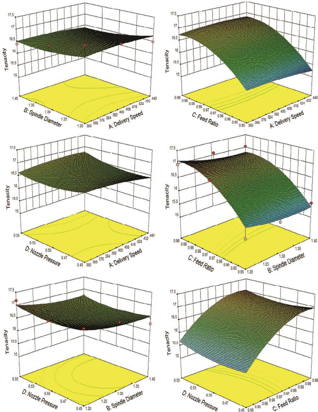
Fig. 1 — Interaction of spinning parameters on tenacity(cN/tex) of Ne 20 polyester/cotton vortex yarn
