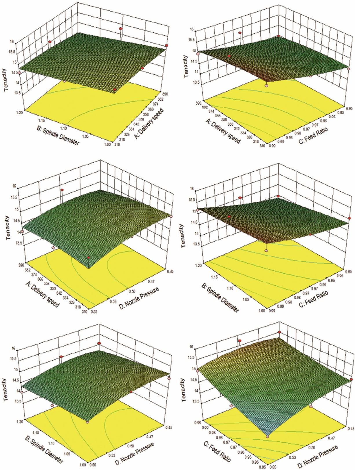
Fig. 2 — Interaction of spinning parameters on tenacity(cN/tex) of Ne 40 polyester/cotton vortex yarn
