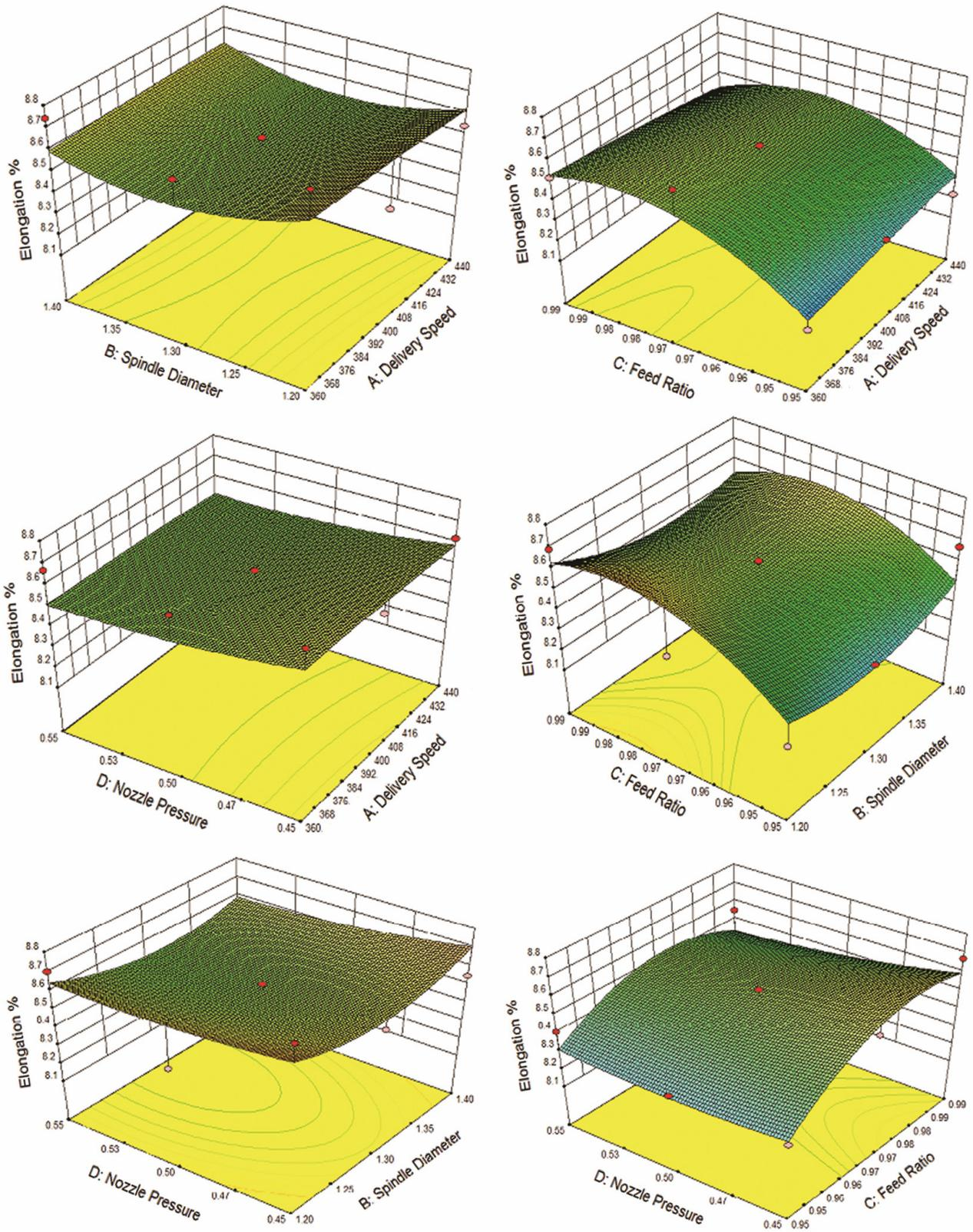
Fig. 3 — Interaction of spinning parameters on elongation of Ne 20 polyester/cotton vortex yarn
