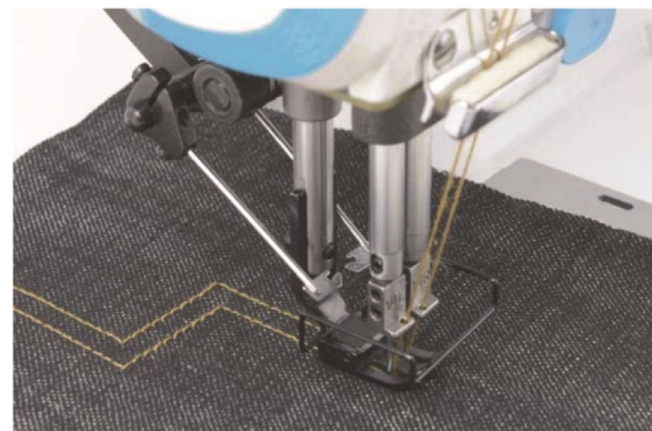
Fig. 1 — Denim fabric under foot pressure during seam process
