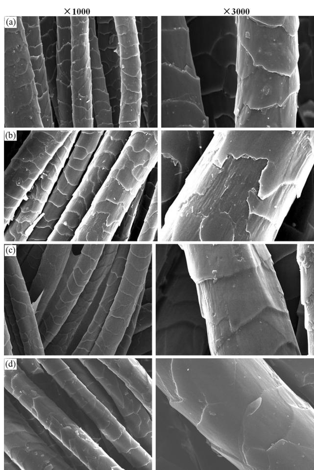
Fig.6—SEM photographs of untreated wool (a), wool oxidized with hydrogen peroxide (b), wool oxidized and treated with CGH (c), and wool oxidized and treated with CGH and CA (d)
