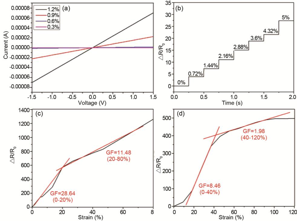
Fig.2 — C-V Curves of sensor (a), resistance change within the low strain range of 0-5% (b), and at different tension in the wale direction (c) and course direction (d)
