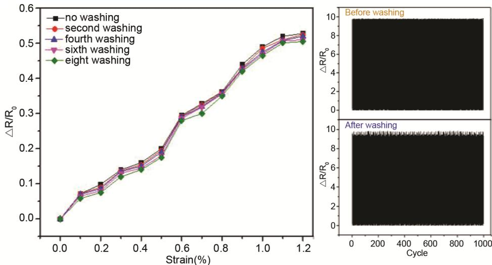
Fig. 5 — Changes before and after washing (a) resistance at different tension and (b) stability when stretched from 0% to 0.2% after 1000 times
