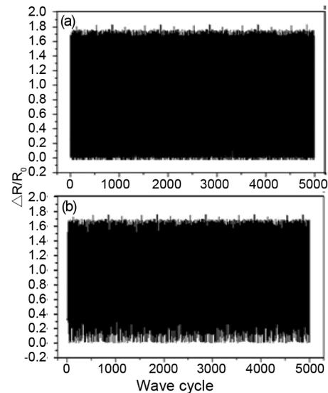
Fig. 3 — Stability stretched from 0% to 0.2% after 5000 times in wale direction (a), and course direction (b)
