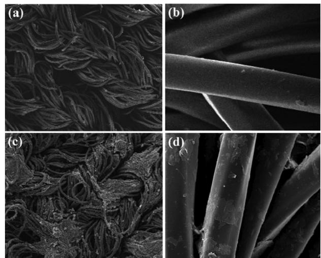
Fig. 1 — SEM images of original fabric at (a)  $\times 100$  & (b)  $\times 5000$ ; and treated fabric (c)  $\times 100$  & (d)  $\times 5000$  magnifications
