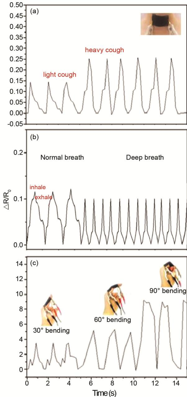
Fig. 6 — Response curves of fabric sensor at different positions (a) light cough and heavy cough, (b) normal breath and rapid breath and (c) bending finger and leg in different angles
