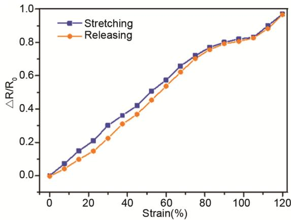
Fig. 4 — Relative resistance under a 120% strain stretching-releasing cycle (strain rate 10%/s)
