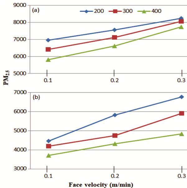
Fig. 3 — Effect on PM<sub>2.5</sub> emission (a) needle punched material and (b) spun bond material
