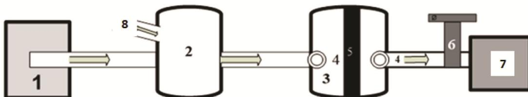
Fig. 1 — Cabin air filter test rig (1- Diesel engine, 2- Dilution chamber, 3- Specimen chamber, 4- Pressure sensor and PM<sub>2.5</sub> meter, 5- Test filter, 6- Suction control valve, 7- Suction motor, 8- Clean air duct)
