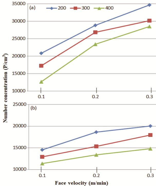
Fig. 5 — Effect on particle number emission (a) needle punched material and (b) spun bond material
