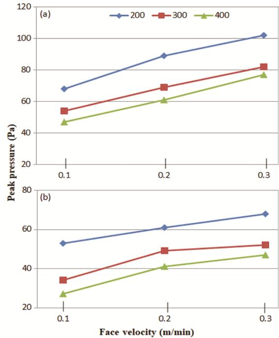
Fig. 6 — Effect on peak pressure (a) needle punched material and (b) spun bond material
