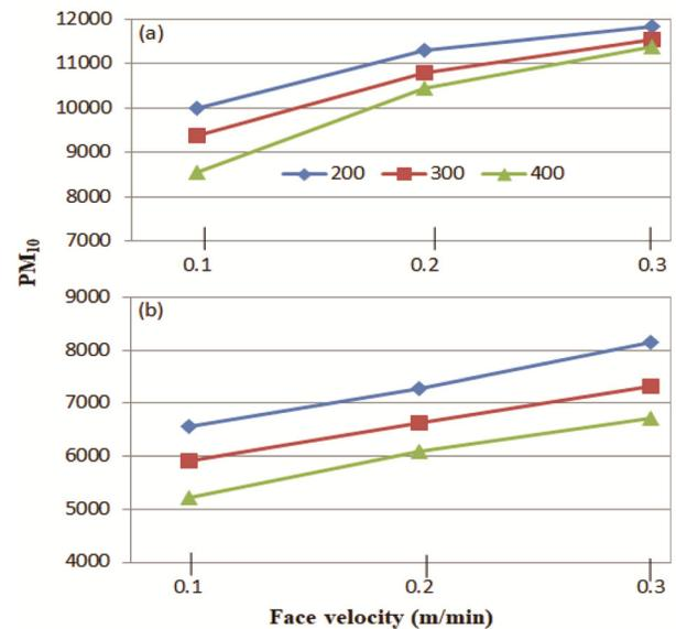
Fig. 4 — Effect on PM<sub>10</sub> emission (a) needle punched material and (b) spun bond material
