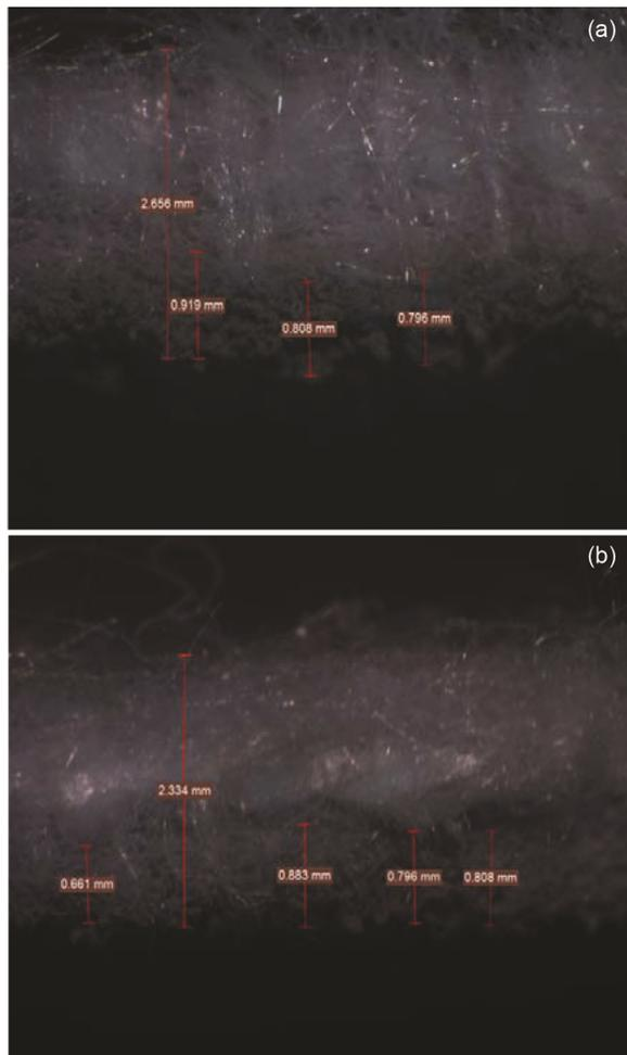
Fig. 7 — Cross-sectional image of tested filter materials (a) spunbond media and (b) needle punched media
